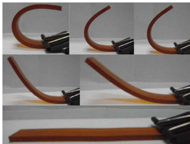
Figure 8. Visual demonstration of shape memory effect for A4. [Color figure can be viewed in the online issue, which is available at wileyonlinelibrary.com .]
